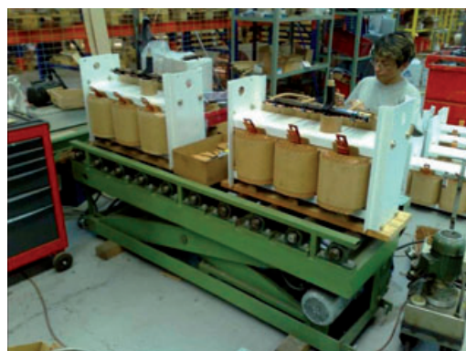
After - automated conveyor of adjustable height.
