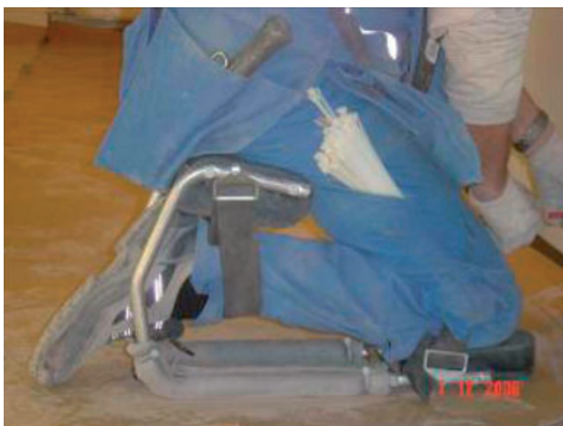
A special device was introduced to protect knees. The device also functions as a stool.
