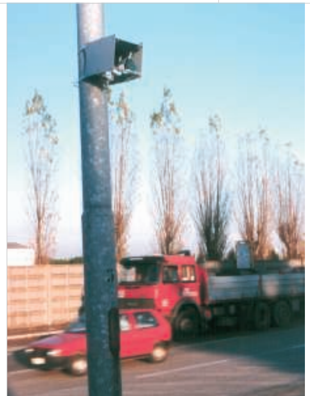
The benzene monitoring device is placed in selected sites around the city.
